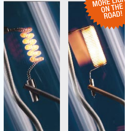
In comparison with standard lamps (left) the Single Coil of OSRAM TRUCKSTAR® (right) offers a visibly more homogeneous light and illuminates the road more evenly and to a greater distance. The clearly improved visibility in the crucial range of 50–100 metres ahead of the vehicle means active protection against accidents and more safety.
